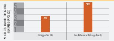
Tested in accordance with ASTM C 1492-03 and performed with low profile, lightweight tile.
