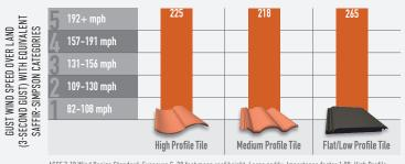
ASCE 7-10 Wind Design Standard. Exposure C, 30 foot mean roof height, Large paddy, Importance factor 1.00, High Profile based on a tile factor of 1,407, 2:12 to 6:12 slope, gable/hip roofs.
