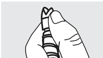
2. Easily snap-off the fan tip to change spray pattern!
