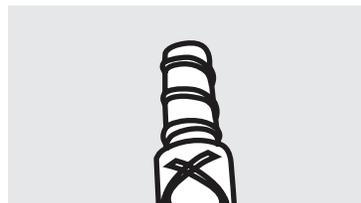
3. Snap-tip nozzle now allows for a cone spray pattern.
